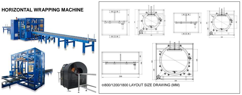
THE EQUIPMENT IS SUITABLE FOR AUTOMATIC WINDING PACKAGING OF SMALL SECTION BAR MATERIALS SUCH AS COPPER, ALUMINUM AND ROUND STEEL.
