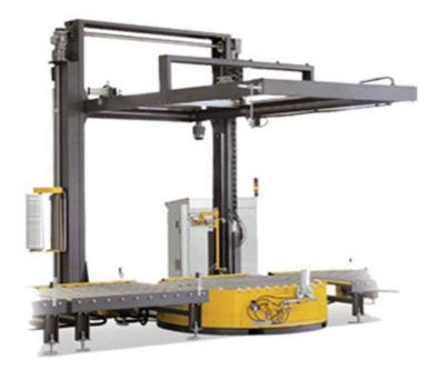
FULL AUTOMATIC PALLET STRETCH WRAPPING MACHINE FOR PRODUCTION LINE AUTOMATIC FILM SEND, AUTOMATIC WELDING FILM, HIGH EFFICIENCY AND SAFETY THE TOP IS COVERED WITH FILM TO REALIZE FIVE-SIDED AUTOMATIC PACKAGING
